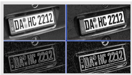
Fig. 6 Result of edge-filtering. Original image (upper left), pre-processing by erosion (upper right), and two different methods of edge extraction, morphological gradient (lower left) and Sobel edge detector (lower right).
