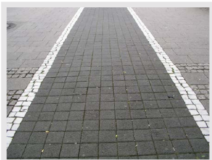
Fig. 4 Perspective distortion with a standard lens. Scale varies significantly through the field of view.
