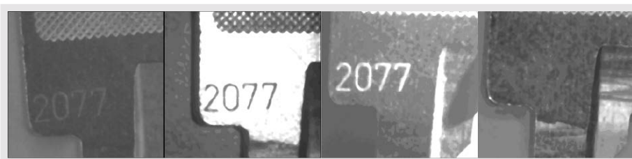
Fig. 2 The same object under different lighting conditions. From the left: Undefined ambient light; bright field lighting; dark field lighting; diffuse light. Contrast between gravure and plain metal can be enhanced or eliminated.
