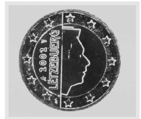
Fig. 3 A coin under directional lighting from an LED-ring. Edges are highlighted.
