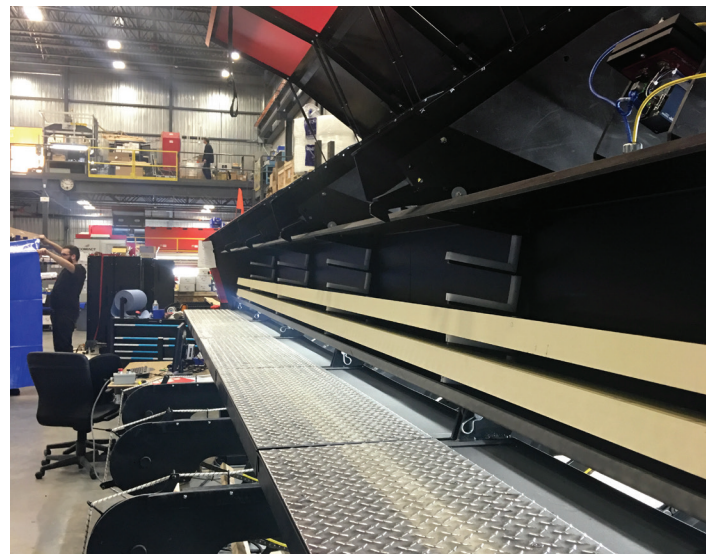
» COMACT's custom-built wood inspection system.
