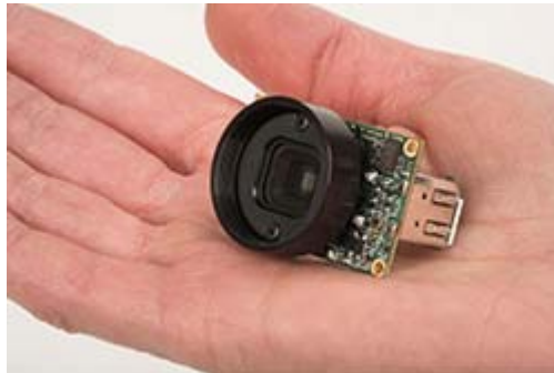
Tiny 29x40mm Firefly MV IEEE-1394 digital camera
