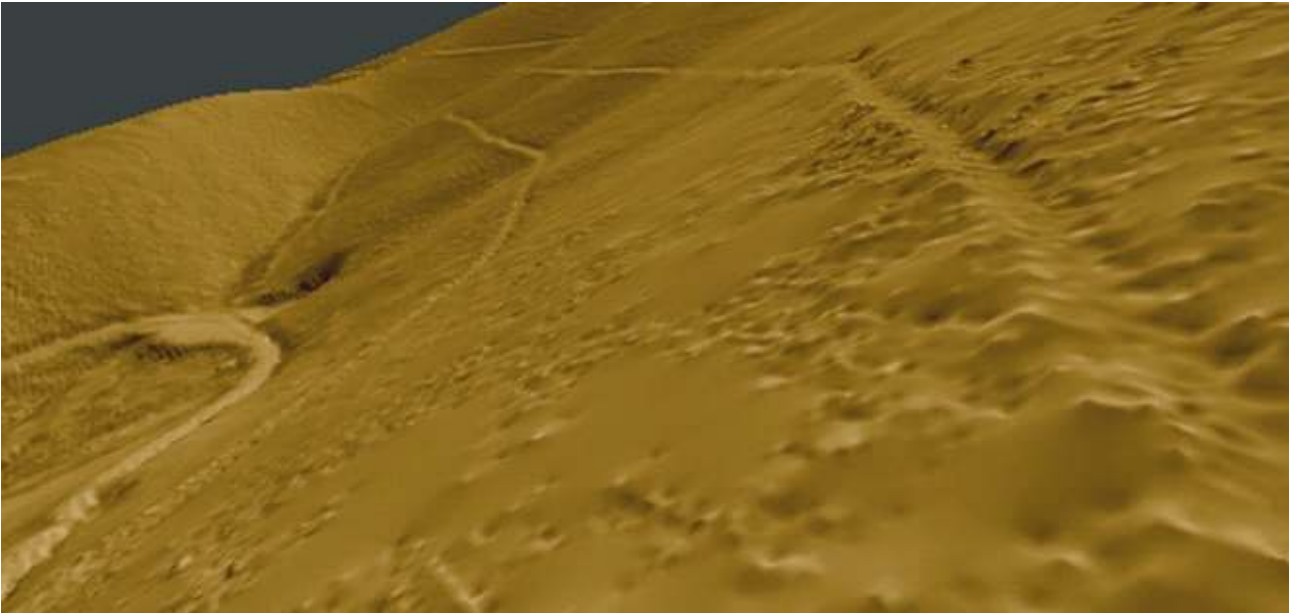
Fig. 2: Digital terrain model (DTM) with clearly visible forest trails.
